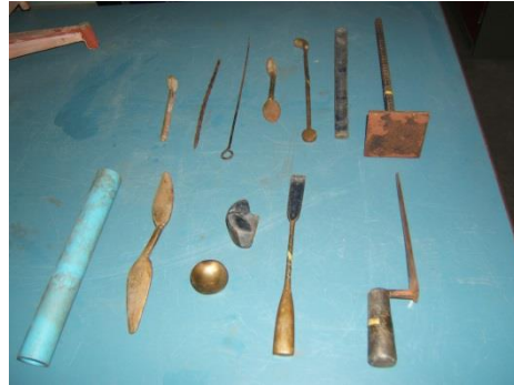
Green sand mold making equipment
