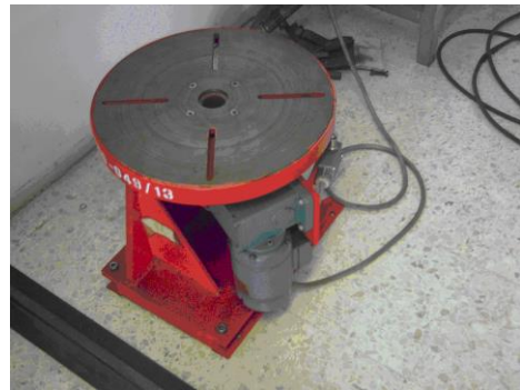
Rotary Table welding fixture
